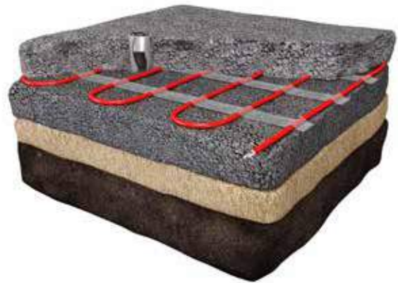
Installation in unrolled asphalt
