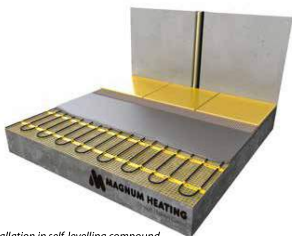
Installation in self-levelling compound
