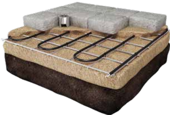
Installation in sand bed under paving stones
